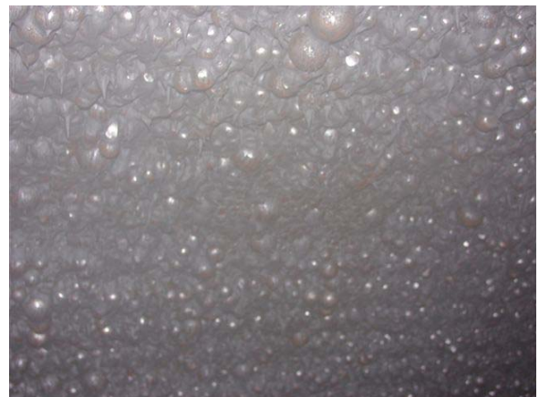
Figure 5. Metal magnetic mill liners with protection layer of ball chips and magnetic minerals (Courtesy of Kevin Berglund).
