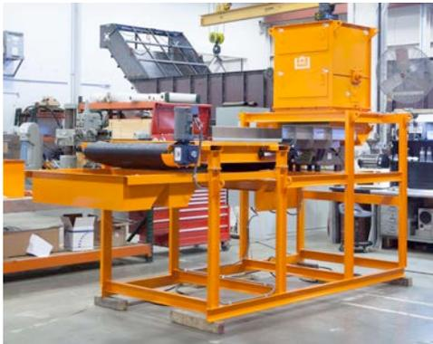
Erie, PA—The new Eriez® [Stainless Steel Rare Earth Roll Magnetic Separator](#) represents a breakthrough for wire chopping facilities, giving users a long-awaited solution to effectively remove stray stainless steel prior to any chopping lines. It reliably recovers and concentrates stainless steel from the “Zurik” conductive fraction from a fines -1” sensor sorting machine or the waste fraction from a fines -1” eddy current separator.
